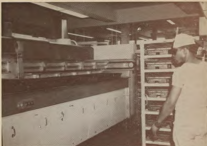
After being in the proof box for 45 minutes, the pans are placed in the oven. The oven holds eight pans across, each consisting of four units. At one time the oven can hold 275 of these pans.
