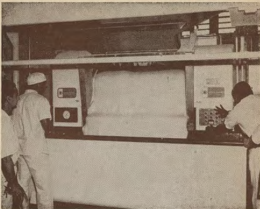
After dough has been mixed, a process lasting 18 minutes, it is placed automatically into a tub that can hold 1,600 pounds of dough.
