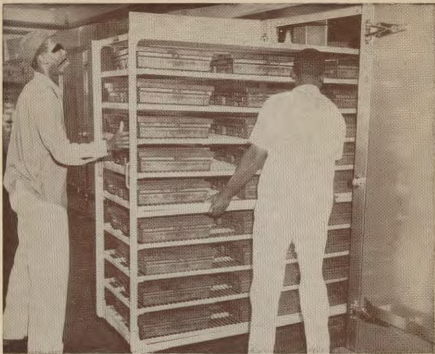
The dough is placed in the proof box for 45 minutes. It is given time to rise before it is placed in the oven.
